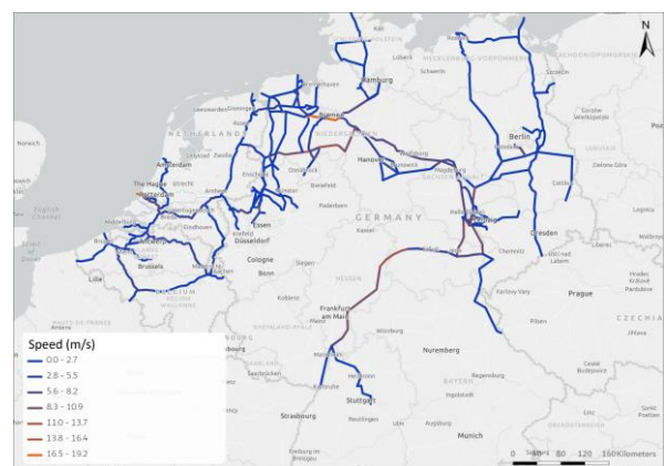
Figure 3.36 Velocity distribution throughout the network for a base network pressure of 40 bar and the 2030 reference scenario.
